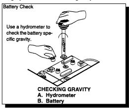
To find the correct specific gravity reading when the temperature of the battery electrolyte is other then 80° F (27° C).
